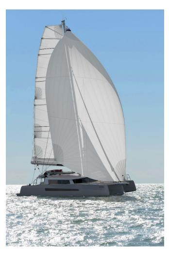
The sail plan comprises a mainsail (with 3 reefs) and a staysail on a rolling furler (on a structural wire inside the sail).
